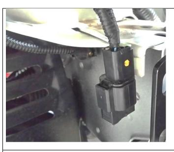
43. Bend small tab retaining plug located on RHS outer chassis rail upwards using pliers (to give better clearance to chassis bracket).
