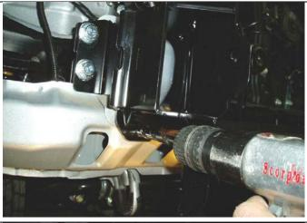
60. Drill Diameter 10mm pinning hole in lower flange of mount bracket into the vehicle Cross member.
