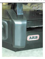
81. Insert the side buffers through the holes and fix using 12x M6 flange nuts.
