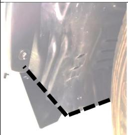
93. Trim sections of wheel arch guard using lower edge of crash beam and wing as guide.
