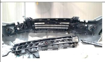
15. Remove the Fog lights, Wiring harness and washer hoses (if fitted) from the back of the bumper and set aside.
