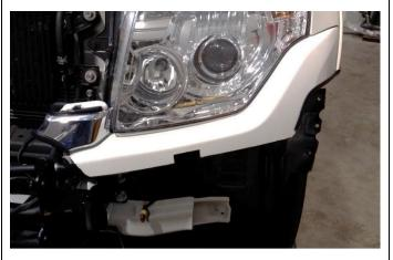
25. Trim bumper and grille along marked edges using a jig saw (apply masking tape to either side of cut lines before cutting).
