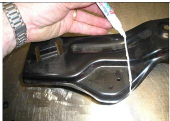
26. Mark cut lines on each end of the cross member. The edge of the cut is 25mm inboard of the M6 hole as shown.
