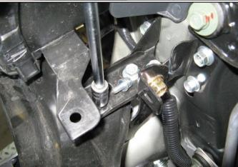
13. Undo upper cross member fasteners as shown on both end.
