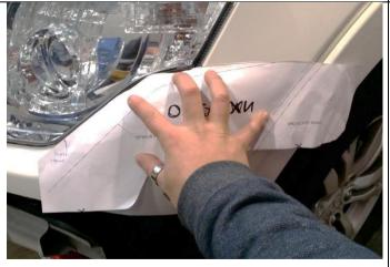
19. Position/align bumper trim template with edges listed on template and mark cut line.
