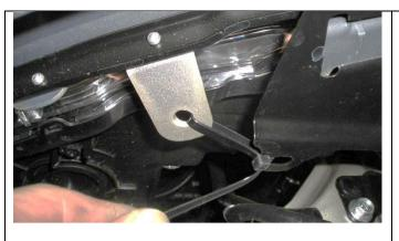
38. To secure inboard end of bumper section, fit a cable tie to the remaining lug on the bumper and through the newly drilled hole in the cross member ends. This cable tie when pulled tighter can adjust the position of the bumper to the bull bar, so wait until after the bar is fitted before trimming the cable tie off.
