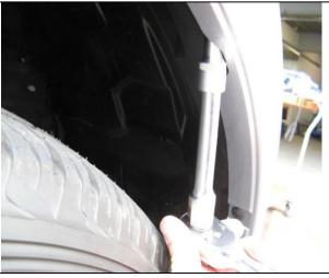
5. Undo vertical screws securing bumper to fender
