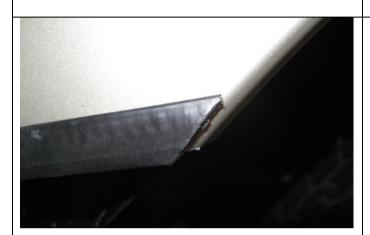
39. Mark and then trim one end of each of the pinch welds to suit the angle of the wheel arch area of the flare. Use a cutting wheel in a grinder as there is a metal spring channel frame inside the pinch weld.
