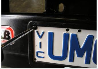
80. Fit number plate using black dome head screws inserted into grommets.
