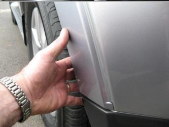
10. Free the end of the flare from the bumper by pulling outward in the lower region as shown.
