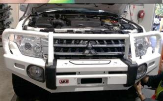
88. Offer bar to vehicle and loosely fasten using 6x M10x30mm SEMS bolts and 6x M10 flange nuts.
