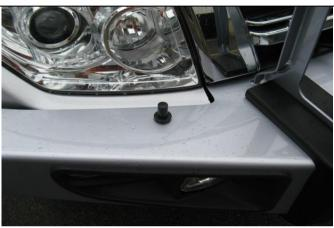
82. Fit Headlight Washers to Bar if required, refer to Washer Kit Fitting Instructions.
