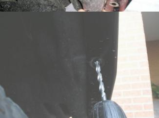
95. Drill holes in fender liner using Φ7.0mm holes in wing return flanges as a guide and fasten fender line with 4 x M6x25mm black bolts, M6 washers, M6 spring ashers and M6 flange nuts.
