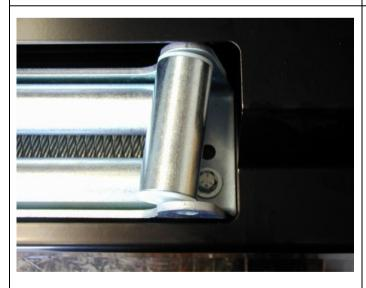
67. Remove the cir clips from the bottom of the vertical rollers of the fairlead and push the pin upwards. Push the vertical rollers inwards on the lower edges as shown and using two 3/8" x 1 3/4" bolts M10 flat and flat washers, attach the lower section of the roller fairlead to the bull bar and winch.
