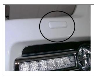
16. If washer assemblies fitted (circled for reference in picture), remove and set aside.
