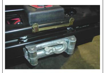
75. Install licence plate bracket to bar using 2x M6 flange nuts, 2x M6x16mm bolts and 2x M6 washers.
