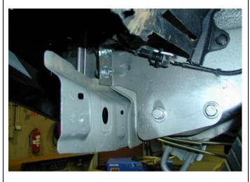
62. Reclip electrical loom connector into new bracket flange both sides of vehicle.
