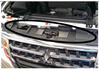
6. Remove scrivets securing grille across the top and pull grille upward to release lower clips.
