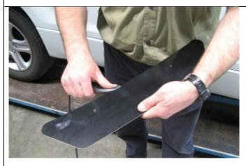
76. Apply rubber mould to edge of winch hole cover panel and trim off excess.
