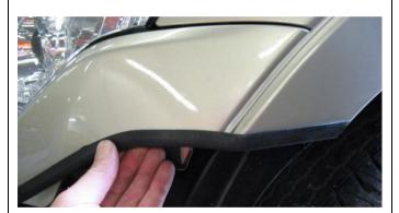
40. Apply pinch weld to both chrome grille piece and bumper (two separate pieces need to be cut).
