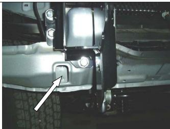
61. Fit M10 SEMS bolt and load flange nut from inside cross member then do up tight to specified torque.
