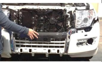
17. Place bumper back on vehicle including securing wing area of bumper into retaining clips.
