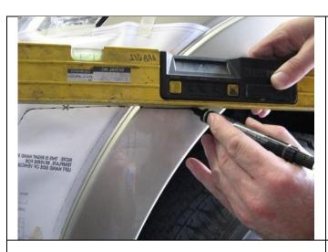
20. Using a spirit level, continue marked cut line onto flare.
