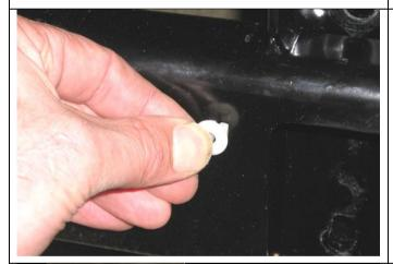
79. Fit 2 x large round head grommets to front face of bull bar in square holes.
