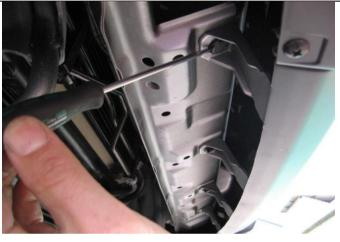
2. Remove plastic scrivets and bolts securing lower bumper tabs.
