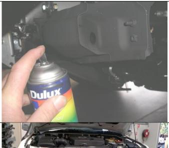
87. Using a black spray pack, paint the exposed colour coded area of the cross beam so it does not show.
