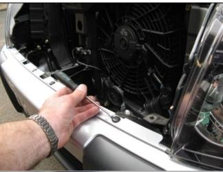
7. Remove upper bumper retaining scrivets.
