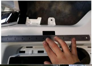
21. Continue marked cut line on bumper as shown using bottom edge of rectangular hole as guide.
