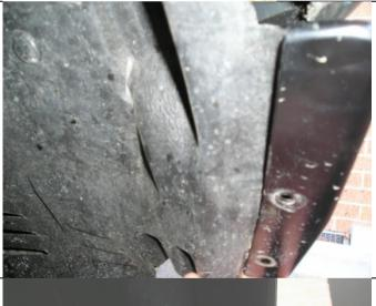
94. Tuck fender liner into inside rear of wing flange.
