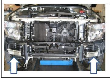
46. Remove metal braces fixing guards to crash beam
