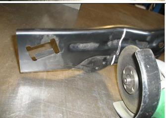
27. Using a jig saw or angle grinder with cutting wheel, cut along the line.
