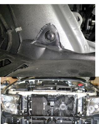
44. Remove scrivet retaining wheel arch guard to outer chassis rail (both sides). This will be trimmed at a later stage.
